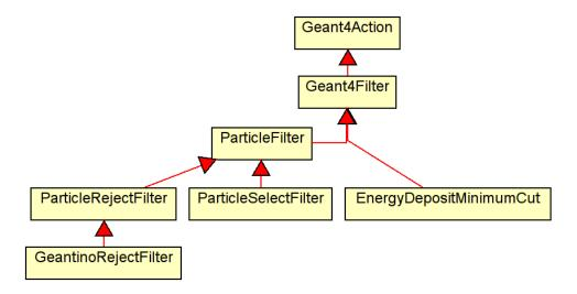
Figure 7: The sensitive detector filters design. The shown class diagram is actually implemented.
