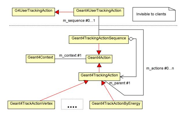
Figure 5: The design of the tracking action sequence. Specialized tracking action objects inherit from the Geant4TrackingAction object and must be attached to the sequence.
