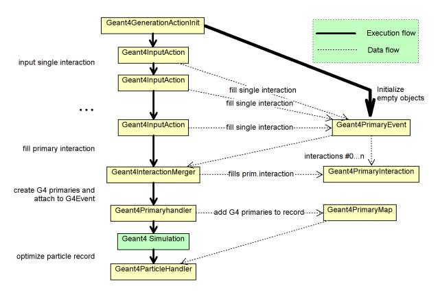
Figure 11: The generic handling of input sources to DDG4.
