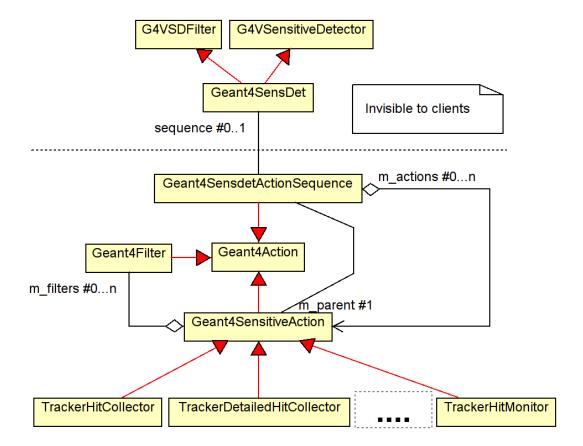
Figure 6: The sensitive detector design. The actual energy deposits are collected in user defined subclasses of the Geant4Sensitive. Here, as an example possible actions called TrackerHitCollector, TrackerDetailedHitCollector and TrackerHitMonitor are shown.
