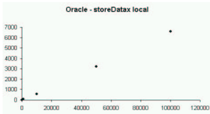
Graph diagram 5 – objects stored vs. time spent storing for Oracle implementation (local)
