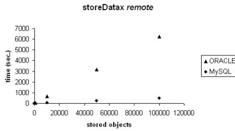
Figure 6: objects stored vs. time spent storing for MySQL and Oracle implementations (remote)
